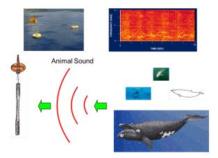
Guide Star Engineering's TASS remote sensor provides reliable data collection, recording, and in-sensor signal processing in real time and for post-processing. Advanced work is being investigated that will give the buoy the ability to automatically detect, classify, and determine the direction and depth of animals.
